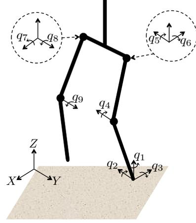
Fig. 1. Robot model with a choice of generalized coordinates when supported on left leg.
